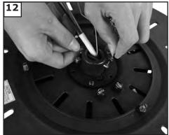
Remove keeper from pin and then pin from yoke and save.
